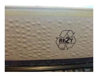
Cockling or honeycomb: too high moisture will cause the fibres to expand. This will happen in proportion a lot more in the width then in the length. The fibre direction of the liner is always perpendicular to the flutes.
