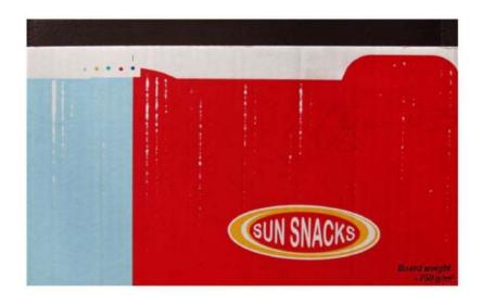
Stripyness caused by post glazing: the corrugating process is a physically very rough process. Take a coated liner, moisten it, heat it and then drag it for about 15 meters under high pressure on metal heated plates. This can and will change the coating structure on the flute tips and will result in a different way how inks are settling or penetrating. You can compare post glazing with what happens if you iron the pants of your best suit too warm...your pants start to shine.
