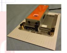
Calculating WBE requires extremely sensitive height measurement while accurate measurements of flatness and flute pitch requires a large area to be measured. These conflicting requirements are solved by the use of sequential image capture and stitching. The CORRCHECK captures 5 high resolution images and creates a compound image over 1.5 inches wide.
