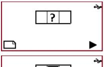
The device is expecting an overprint color measurement of red, green or blue color while a simple color has been measured. The composing colors can not be calculated. Measure an overprint color.
